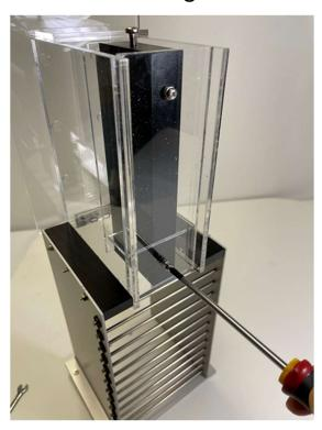
**Note:** to avoid damage to the acrylic Staircase Housing walls, only a light tightening torque is required – approximately 1 Nm is sufficient).
