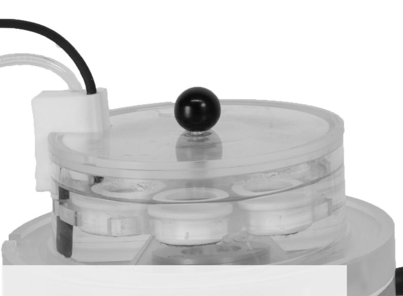
Temperature Controlled *In Vitro* Slice Holding Chamber
