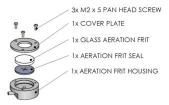
The Glass aeration frit will from time to time require replacement. The frit and seals are available from Campden Instruments (see spare parts and consumables). To replace the frit:
